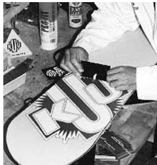
Picture # 9 scraper Removing excess material
