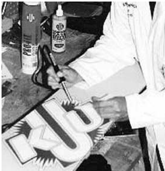
Picture # 8 using Pro-Fix base repair tool
